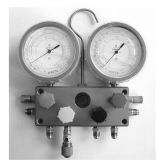
Fig. 7-10 Service gauge manifold
